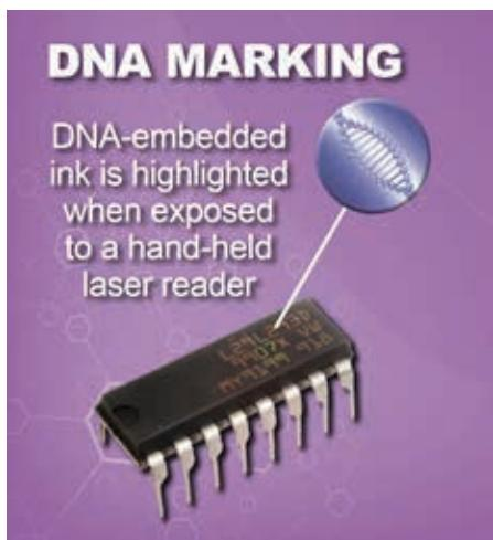
DNA marking consists of applying a DNA identifier to the surface of a microcircuit. A unique code, which can't be replicated, re-engineered or digitally copied, is incorporated into the ink of the DNA mark.
