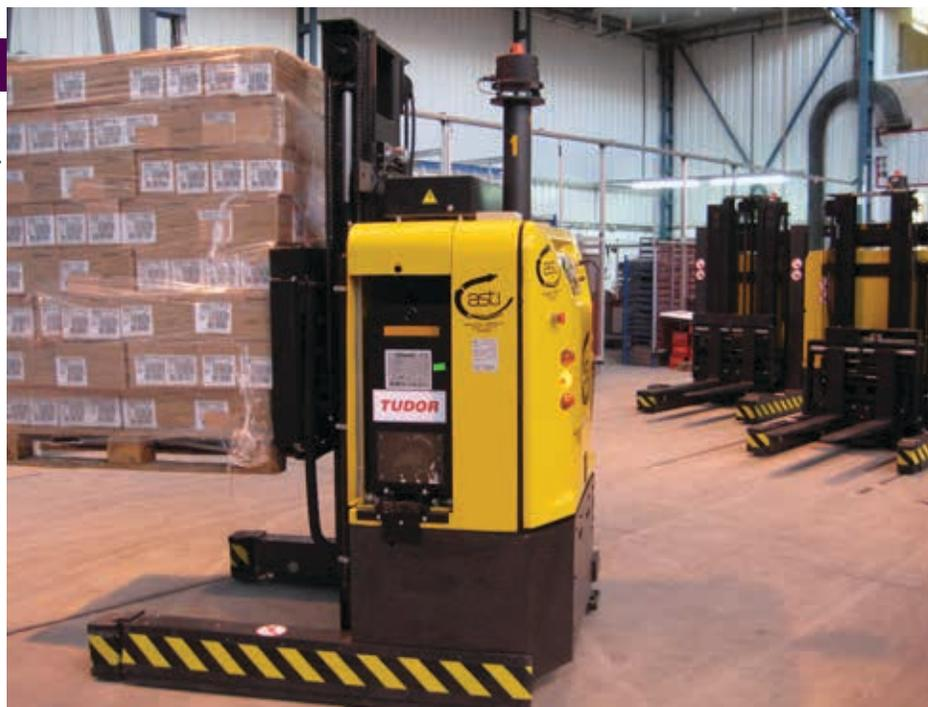
Autonomous guided vehicles can be small and used for maneuvering in tight spaces.
