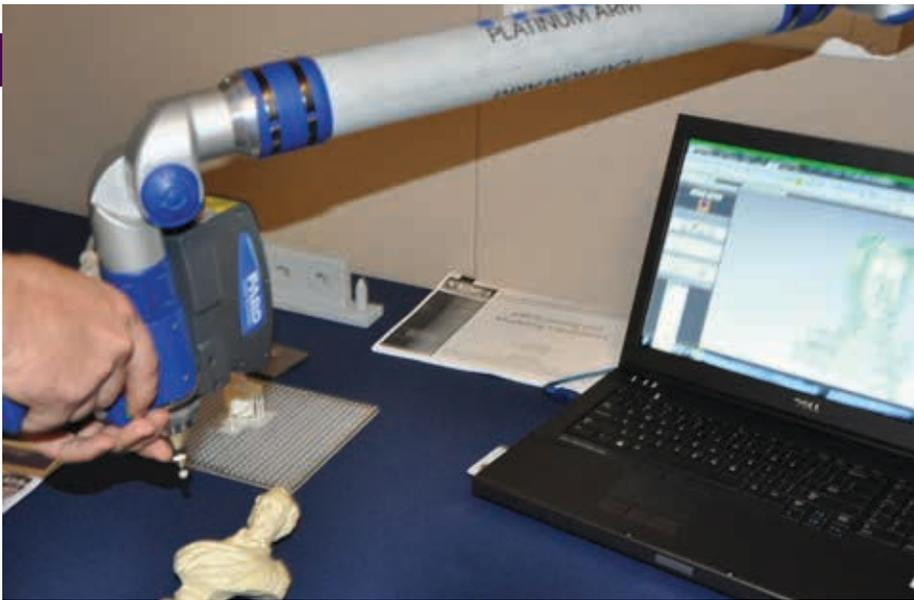
A Navy instrumentation engineer demonstrates how the 3D ScanArm scans objects and creates digital models for printing. The reality of 3D printing is expanding across the Navy's science and engineering community.
