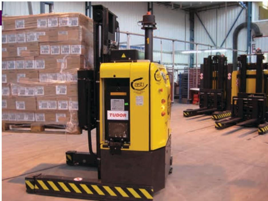
Autonomous guided vehicles can be small and used for maneuvering in tight spaces.
