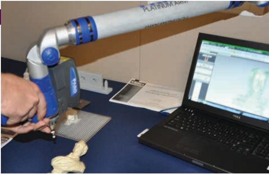
A Navy instrumentation engineer demonstrates how the 3D ScanArm scans objects and creates digital models for printing. The reality of 3D printing is expanding across the Navy's science and engineering community.
