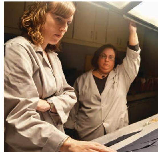
can be done via the human eye or with a color-measuring device. Industry and DoD agree the latter are not adequate for multi-colored fabric, such as camouflage, but industry has become more reliant on devices to evaluate shades for solid-colored fabrics.
